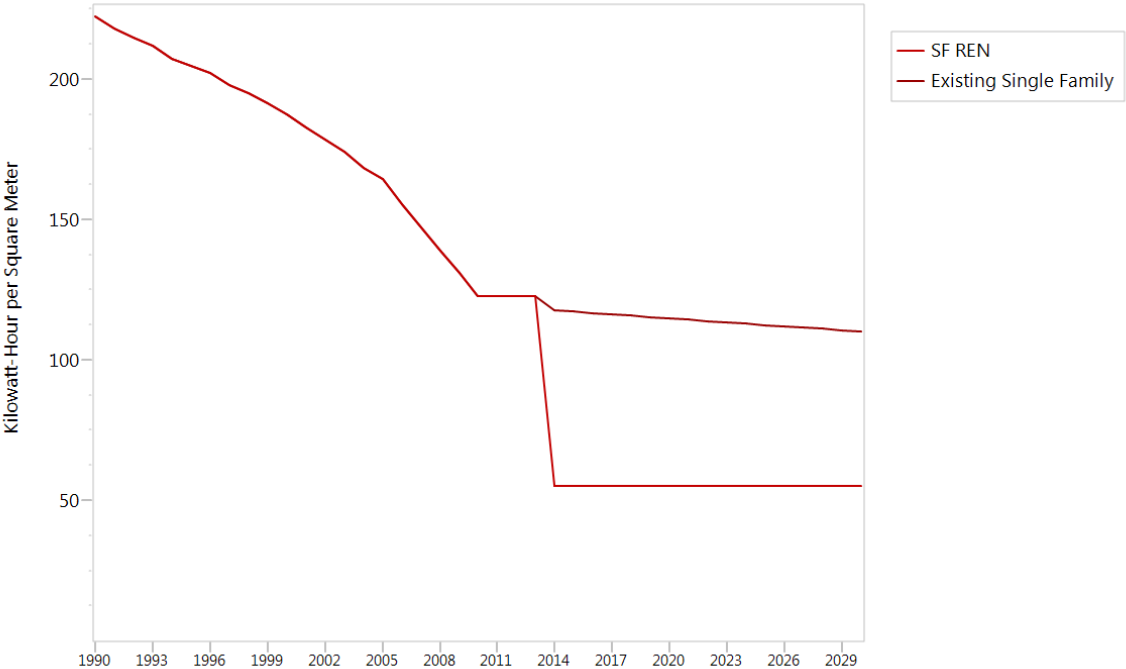
Figure 10: Existing Single Family, Useful Energy Intensity for Space Heating (Kilowatt-Hour per Square Meter).
